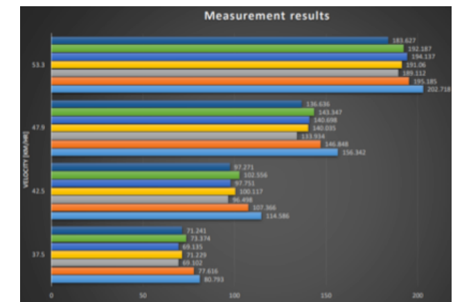
Figure 4 measured drag (in watt). Light blue gives baseline drag without NAQI aero speed gel. Other colors are the results different prototypes with changing vortex generators inside the gel.
